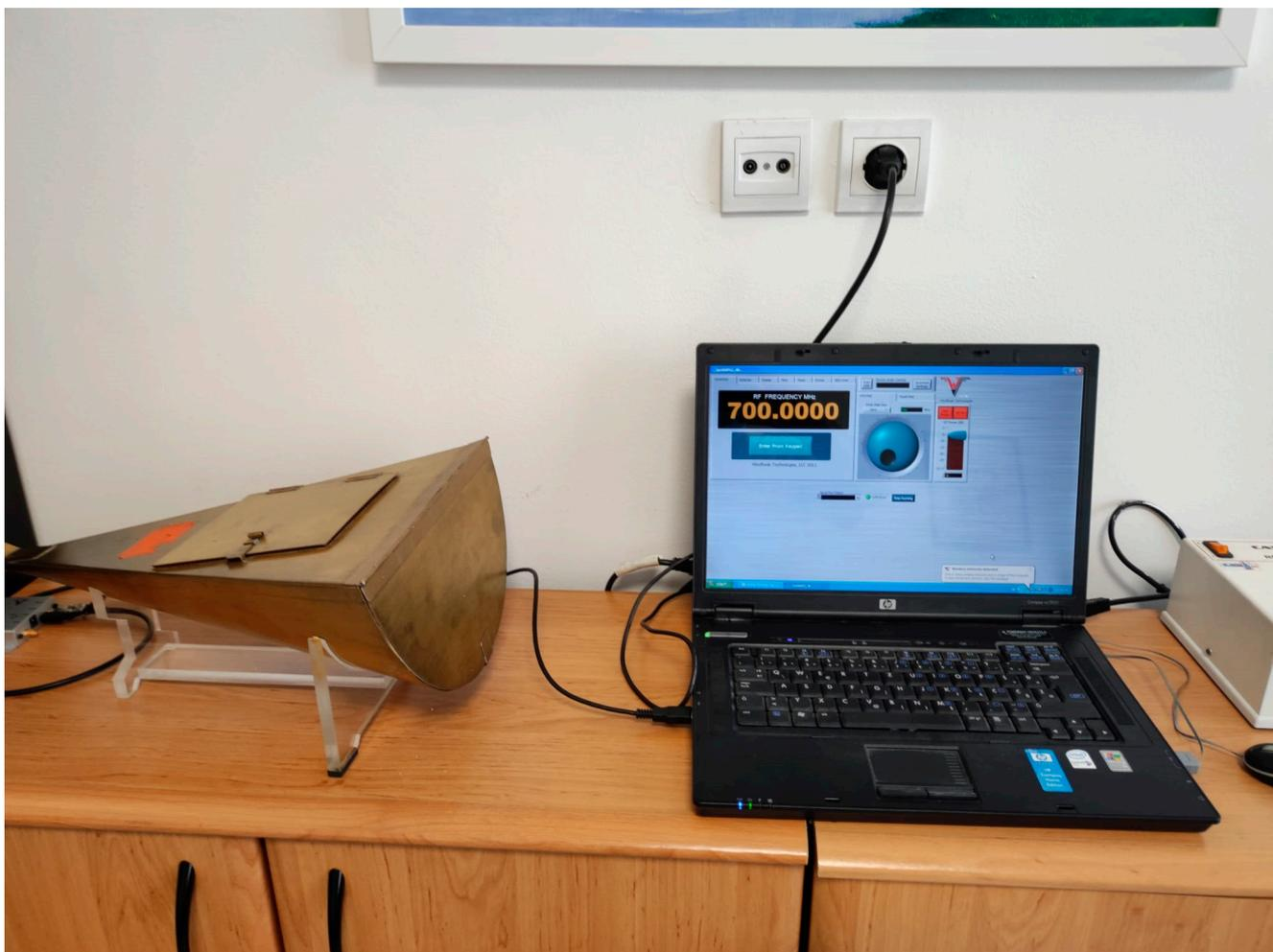
**Figure 1.** Half-cone gigahertz transversal electromagnetic cell and signal generator operated by a laptop.
